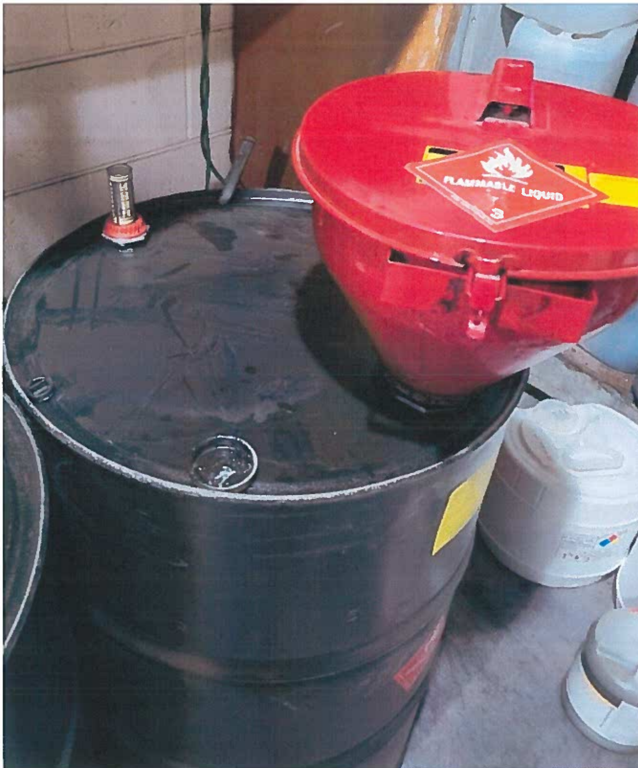
Photo displays the grounding wire clamp, volume gauge and the funnel
