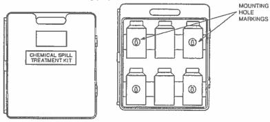
The mounting hole markings can be drilled out to allow either permanent wall mounting or to create 'keyhole slots' for Klt removability. Under normal conditions only the top two markings need be used. Drill a 3/16 in. (4.8 mm) hole in the top of each marking for permanent wall mounting. To create 'keyhole slots,' drill additional 7/16 in. (11.1 mm) holes as indicated below and cut out the material between the small and large holes.
