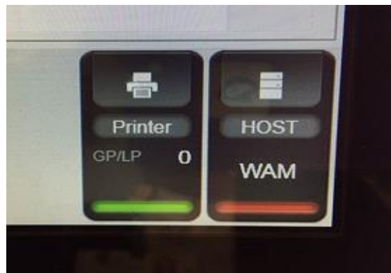
Figure 8: Wam Connection Status is RED. This mean that WAM server is down.
