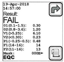
If the EQC Device result is "FAIL", repeat the EQC. If the result is "PASS", continue with patient testing. If the EQC result is
