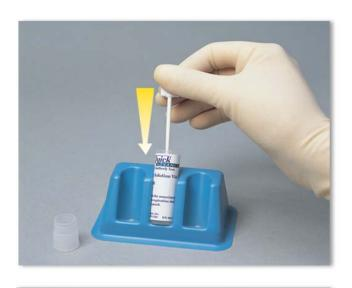
Immerse Loop into Developer Solution Vial.
