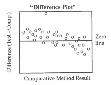
"Difference Plot" - are used if the two methods are expected to show one-to-one agreement. The differences should scatter around the line of zero differences, half being above and half being below the line.
