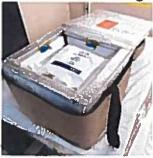
4.4 Obtain the frozen panel from the freezer and place on the top. This must be placed on the top and should not come into direct contact with the units (thus the gel pack)
