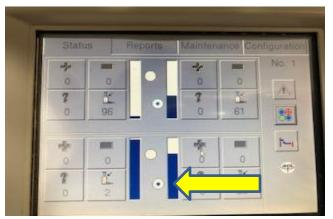
The blue dot indicates the instrument is reading. Pick a drawer that does not have a blue dot in the white circle.
