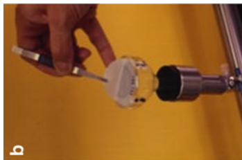
(b) Carefully lay the filter onto the filter-holder base.
