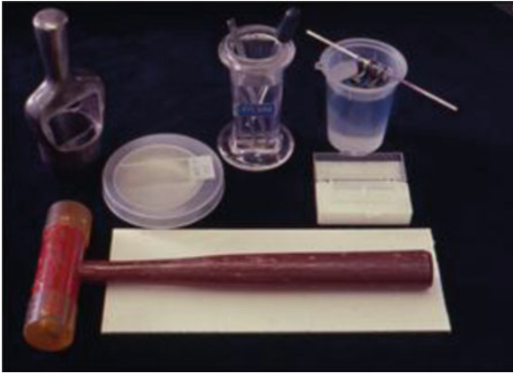
FIG. 18.1. The materials to halve and mount cellulosic filters as shown here simplify the process. They are more than a casual user needs.
