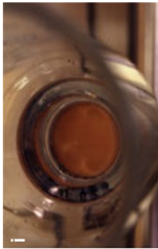
FIG. 7.2. (continued) (i-before) Before alcohol is added to the dilution reservoir, blood is obvious when present.
