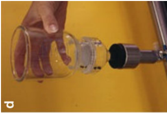
(d) Center the filter-holder funnel on top of the filter-holder base.
