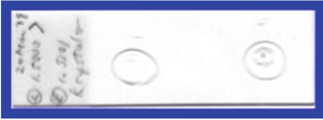
FIG. 16.9. This slide has glass powders with refractive indexes of 1.5000 on the left and 1.5101 on the right. A few drops of the same mounting medium have been added to each area. The slide was oven-dried. The glass particles were then examined microscopically using the Becke line test to determine the 0.01 refractive index window within which the dry mounting medium falls.
