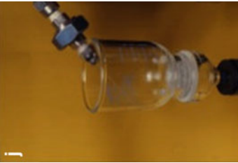
FIG. 7.2. (continued) (j) Never let the filter dry out. Add filtered alcohol to the inside wall of the filterholder funnel. This anchors the cells to the filter. See (j-after).
