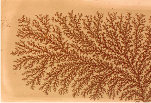
FIG. 18.12. “Ferning” in cellulosic filters results from mounting techniques that don’t compensate for the filter’s 84% porosity.
