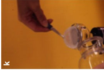
(k) Quickly remove the filter-holder. Using flat-tip forceps, remove the filter and immerse it in alcohol as in (a).
