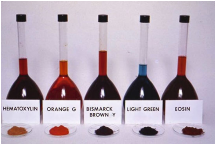
FIG. 10.1. The five dyes that comprise the Papanicolaou stain are in three solutions. Hematoxylin and orange G are each in separate solutions; the third solution EA contains Bismarck brown Y, light green SF yellowish, and eosin Y. I used to prepare aqueous stock solutions in volumetric flasks, as shown, to control the molar concentration of the counterstain dyes.
