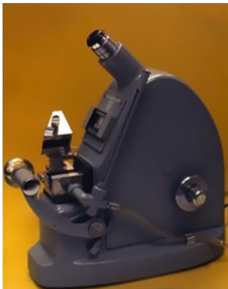
FIG. 16.7. The refractive index of a mounting medium for the D line of sodium was determined directly by using this Abbe refractometer.
