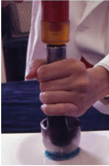
FIG. 18.4. Wipe off the cutting edges of the punch before using it with another specimen.
