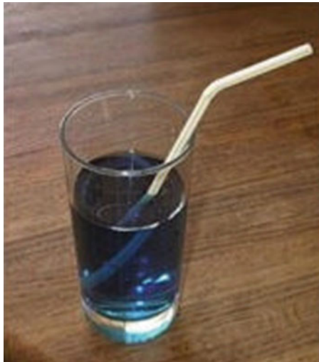
FIG. 16.6. Refracted light “breaks” the straw at the interface of air (RI=1.000) and water (RI=1.333).
