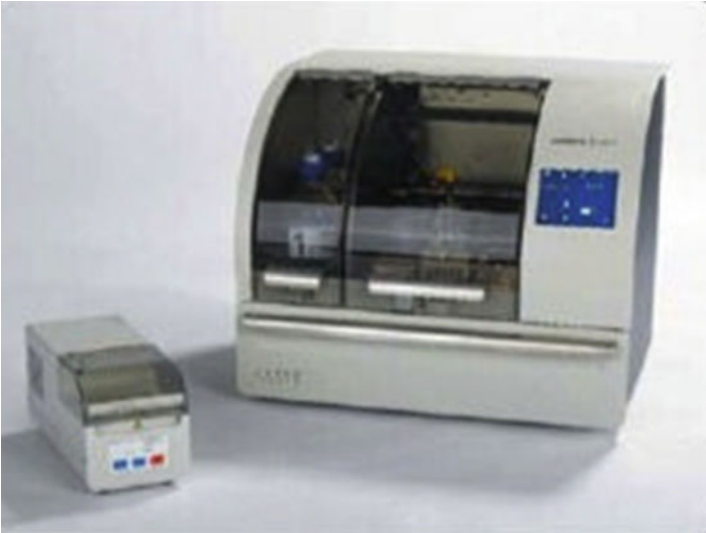
FIG. 9.3. The Cellient automated cell block system processor and finishing station. 12
