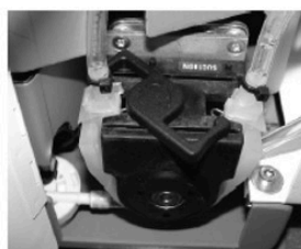
Pump with loosened tubing holder.
