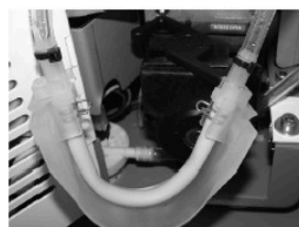
Tubing and holder freed from pump.
