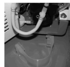
Tubing removed from holder.
