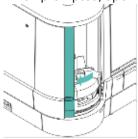
j. Remove the diluent rack and close the load station door.
