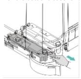
f. Remove the liquid container from the system. Remove the 2 bottle caps. Dispose of the residual liquids in a "dirty" sink.
