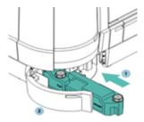
o. Open the liquids door and pull the bottle release for the liquid waste. Remove the liquid waste bottle from the system.
