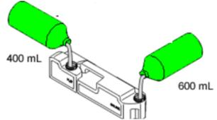
h. Install the bottle caps and gently tilt side to side. Push the bottle back into the system with the bottle insertion tool until it snaps into place. Close the door. The system will perform the decontamination.
