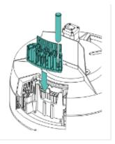
x. Close the load station door. When prompted, open the load station door. Remove the sample rack and sample tube.
