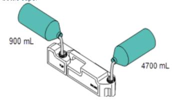
n. Push the bottle back in with the bottle insertion tool, until it snaps into place. Close the door.
