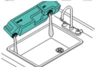
m. Fill the smaller bottle (blue) with approximately 900 ml deionized water and the larger bottle (white) with approximately 4700 ml of buffered saline. Install the bottle caps.
