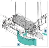
p. Remove the bottle cap and dispose of the liquid waste.
