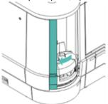
w. Remove and empty the sample tube. Place the empty sample tube back into the sample rack at position 1.
