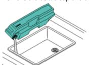
s. Install the bottle cap and push the liquid waste bottle into the system with the bottle insertion tool until it snaps into place.
