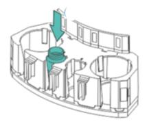
d. Place a new 5 mL of 7% BSA into position 2 of the same diluent rack as the NaOH and load the diluent rack on to the instrument. Make sure there are no bubbles present in the BSA and that the reagent has been brought to room temperature prior to use (bubbles can be mistaken as clots by the instrument during daily QC).
