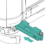
e. Pull the bottle release for the liquid container.
