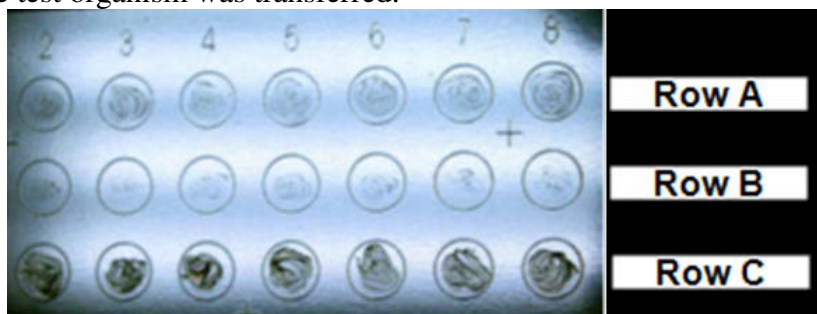
Ideal (row A) and suboptimal (rows B and C) amounts of test organism on a target
