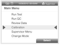
Following the prompts, insert the Calibration Cassette into Sofia and close the drawer. Sofia performs the Calibration Check automatically with no user input required.
