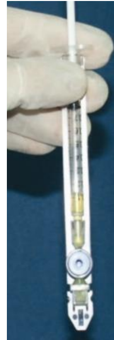
Figure 3 Inspect for bubbles
