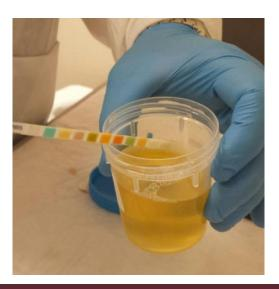
Do not to bend the strip while sampling. A bend in the strip may cause it to get lodged inside the analyzer and prevent it from working.
