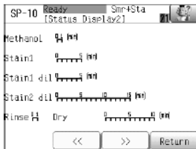
Figure 32 – SP-10 Staining Process Status Display Screens
