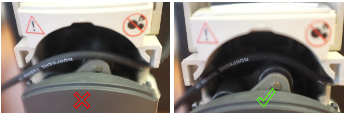
Fig. 5. Position of the tube in the peristaltic pump
