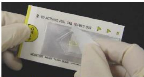
3. Grip where indicated. Lift up silver tab so that white developer pad is visible.
