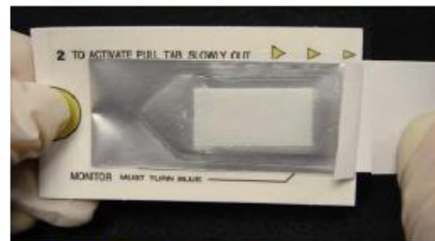
4. Pull silver tab SLOWLY all the way to the right and completely remove it. Developer pad will "flip over" as the tab is pulled.
