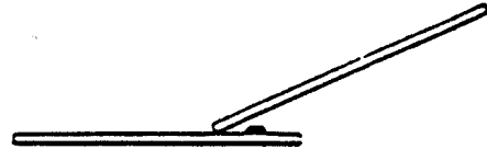
Fig. 117. Proper 25° angle for spreader slide.
