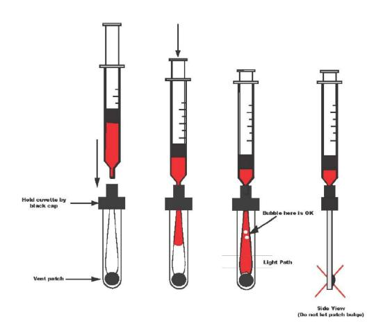
7. Remove any sample on the cuvettes exterior surface before inserting into the GEM OPL.
