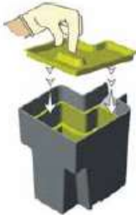
Installation of the disposable bin cover
