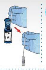
Recap the Sample Reagent vial and vortex for 10 seconds.
