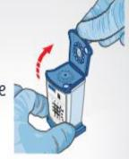
Aspirate all of the Sample Reagent vial contents with a disposable transfer pipette.
