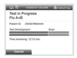
For example: This display shows that the test in Walk Away mode has 12 minutes, 13 seconds remaining. The Sofia Analyzer will read and display the results after 15 minutes.
