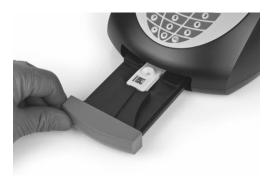
5. Upon closing the drawer, the Sofia Analyzer will start automatically and display the progress, as shown in the example below. In the Walk Away Mode, the test results will be displayed on the screen in approximately fifteen (15) minutes after the Cassette is inserted into the Sofia Analyzer. In the Read Now Mode, the test results will be displayed on the screen within one (1) minute, after the Cassette is inserted into the Analyzer. See Interpretation of Results section.
