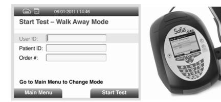
2. Press the Down Arrow on the Sofia Analyzer keypad to go to the Patient ID or Order # field. Input patient ID or Order # using the barcode scanner or manually enter the data using the key pad.
