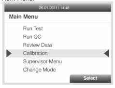
Following the prompts, insert the Calibration Cassette into the Sofia Analyzer and close the drawer. The Analyzer performs the Calibration Check automatically with no user input required.
