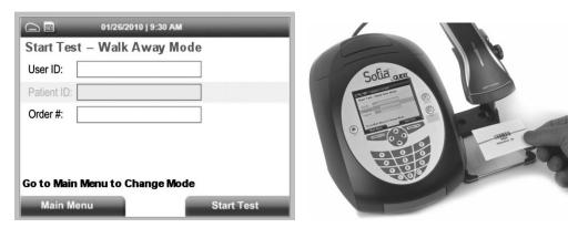
3. Press Start Test and the Sofia Analyzer drawer will automatically open.
