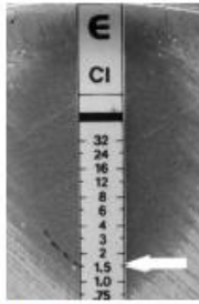
Figure 12. Bactericidal agents; read at complete inhibition of hazes and microcolonies. MIC 1.5 µg/mL
