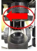
Open the iris aperture completely by turning to the left
