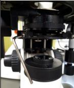
Using centering screws, move focal point to centre of field. Use an allen key
