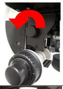
Rack the condenser all the way up by turning counterclockwise
