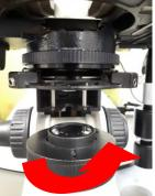
Open the field diaphragm (turning counter clockwise) until the focal point (bright portion) is just filling the field. The dark outline should be just outside the field
