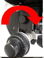
Lower condenser by turning clockwise until the edges of the focal point are crisp
