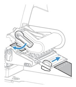
8. The media is automatically advanced once you lock the printhead in place.
