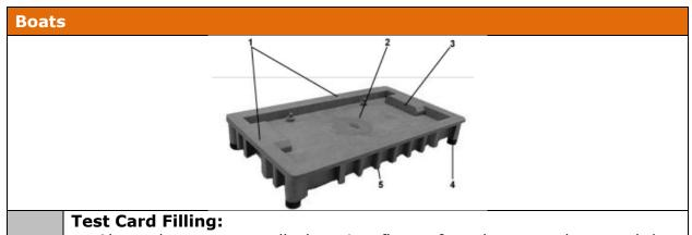
Above the cassette well, there is a flat surface that extends around the perimeter of the boat. This surface becomes the base of the vacuum chamber when the boat reaches the Filler station
