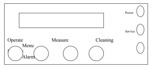
**Standby** – This mode is displayed when the system is not operating any of the internal components. Normally this mode is used when starting a maintenance procedure. The system performs an automatic flush of the RO cartridge every 6 hours (all operating modes). The flush mode rinses the RO to remove anything that has built up on the membrane surface. No water will be sent to the analyzer when the system is in this mode.
