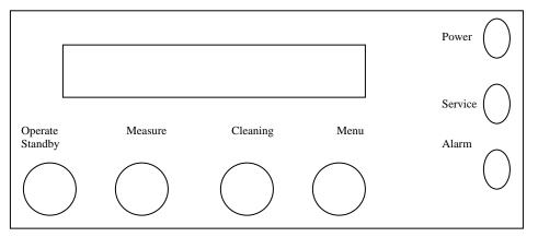
**Standby** – This mode is displayed when the system is not operating any of the internal components. Normally this mode is used when starting a maintenance procedure.
