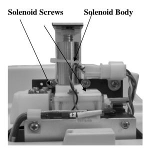
i. Return the cleaned solenoid plunger, including spring, retainer and any washers, to the solenoid body. Secure the retainer and remove the chamber cleaner.
