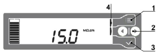
**1 – MODE key** – This button is used to switch between different system modes: Standby or maintenance mode, Ready or tank filling mode and Configuration mode.
