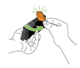
5. Using the color-coded letters for help, slide the ink cartridge into the empty slot until it clicks securely into the slot.
