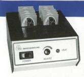
Please note: The indicator must be heated (to 38-42°C for 60 seconds) and placed on a refrigerated blood bag (between 1-3°C) for proper activation.
