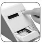
Press the DATA button on the analyzer once or twice (depending on the test cassette) to view remaining results.
