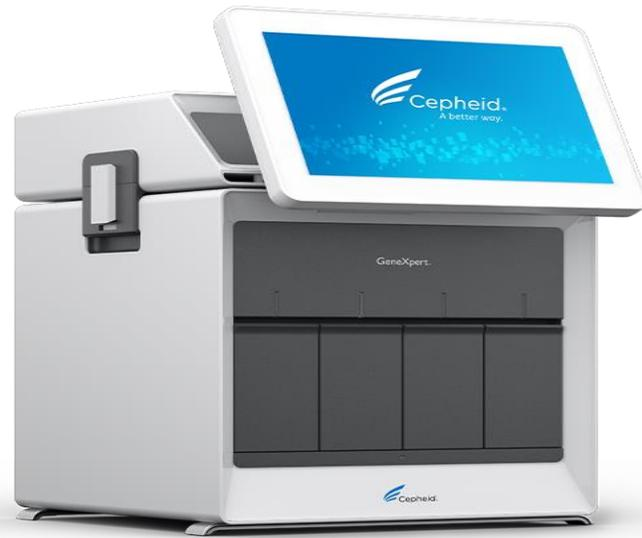
The system is made up of the top screen and barcode scanner and the bottom GeneXpert system. On/Off switches are found on the top front and on the top and bottom of the back of the system.
