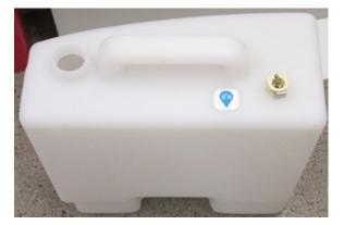
6. Open the water bottle lid and load water bottle onto Centaur. Attach water fitting to bottle.
