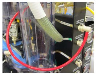
7. Empty the D.I. Water Canister and D.I Water Reservoir. You may need to remove the canister holder because the length of the float switch will prevent you from removing the canister. Loosen canister from lid first with canister wrench then loosen the 4 mounting screws.
