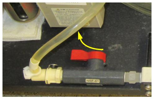
5. Using the red bypass tubing, with the quick disconnect fittings on both ends, plug one end into the Main Vacuum Check Point female connector.
