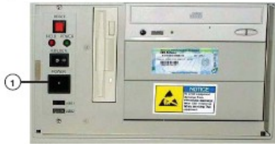
Figure 5.12: Input/Output module computer power switch
