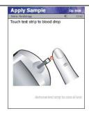
Note: the test strip must fill completely after touching the blood droplet. If the test strip does not fill completely, do not touch the blood droplet a second time. Discard the test strip and repeat the test with a new test strip.
