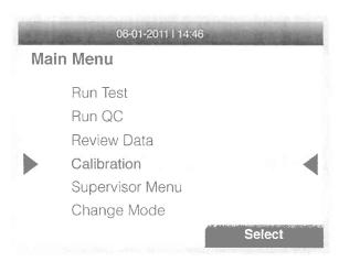
2. Following the prompts, insert the Calibration Cassette into Sofia and close the drawer. Sofia performs the Calibration Check automatically within 2 minutes with no user input required.
