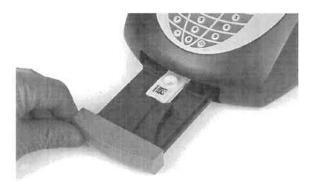
5. Sofia will start automatically and display the progress, as shown in the example below. In Walk Away Mode, the test results will be displayed on the screen in approximately 15 minutes. In Read Now Mode, the test results will be displayed on the screen within 1 minute. See Interpretation of Results section.
