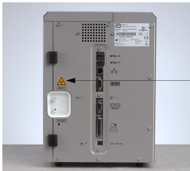
Figure 8.3 Waste Outlet Biohazard Label
