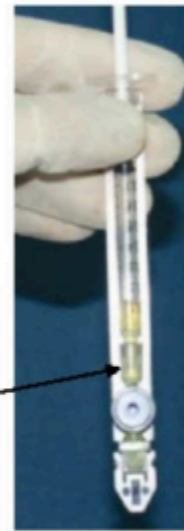
Figure 2: Fill the capillary until the sample appears above the Luer adaptor. Inspect for air bubbles in the capillary and cuvette sections.
