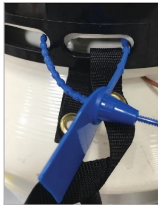
Figure 8. Example of sealed dewar (current generation)
