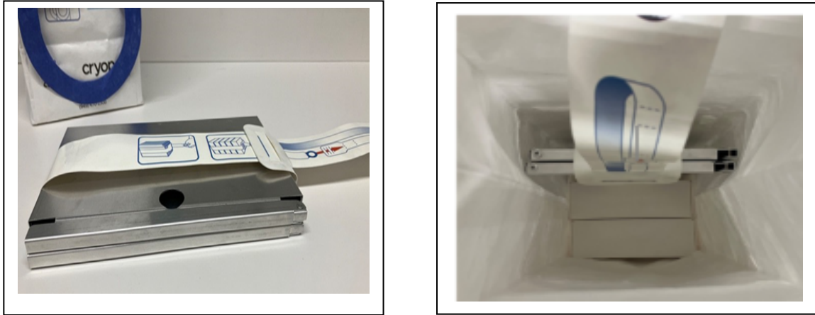
Figure 1. Cassettes wrapped with cryostrap and placed in the Safepak
