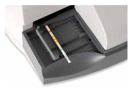
9. Place the strip to the right and parallel to the push bar. Ensure that the end of the strip is against the back wall of the platform and that it is not touching the bottom of the strip loading station.
