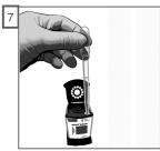
Slowly empty the pipette into the sample chamber of the cartridge
