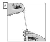
Pipette at least 1 mL of the sample using the provided pipette\*
