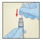
While holding the swab in the same hand, unscrew the cap from the Xpert Swab Transport Reagent tube.
