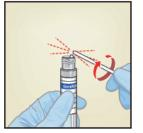
Carefully break the swab shaft against the side of the tube at the scoreline
