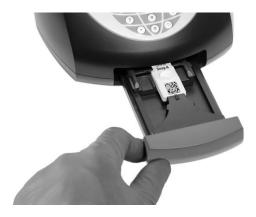
5. Sofia will start automatically and display the progress as shown in the example below. In WALK AWAY Mode, the test results will be displayed on the screen in approximately 5 minutes. In READ NOW Mode, the test results will be displayed on the screen within 1 minute. See Sofia Interpretation of Results section.
