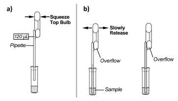
10. Empty the contents of the Pipette into the Test Cassette sample well by firmly squeezing the top bulb. Extra liquid left over in the overflow bulb should be left behind.
