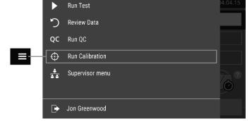
2. Following the prompts, insert the Calibration Cassette into Sofia 2 and close the drawer. Sofia 2 performs the Calibration Check automatically within one minute with no user input required.
